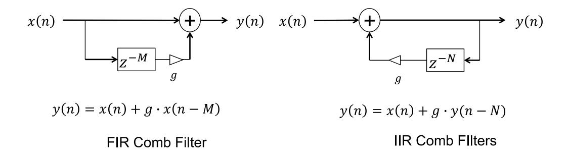
• Implemented by circular buffer: move read and write pointers instead of shift all samples in the delayline
